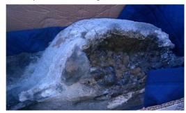
The photo above, taken by Paul, shows the fault point that had to be cut out. The low fault current meant the upstream circuit breaker or fuse didn't "see" enough current to stop the energy flow quick enough, allowing the arc to persist and convert the sand to glass. This situation highlights
