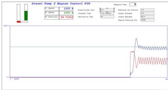
Oscillating Engine Speed During the Tuning Process
