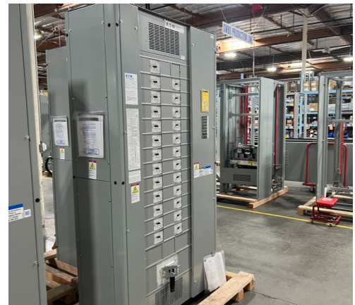
Panelboard Assembly Line – Final Product
